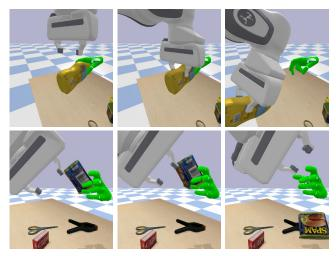
Fig. 3: Simulating objects released from human hands. A release is triggered at the middle frame in the top and bottom examples.
